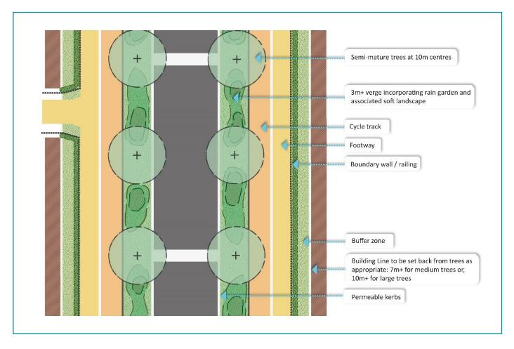
Figure 1: Illustration of an acceptable street tree layout on a Strategic Route.
