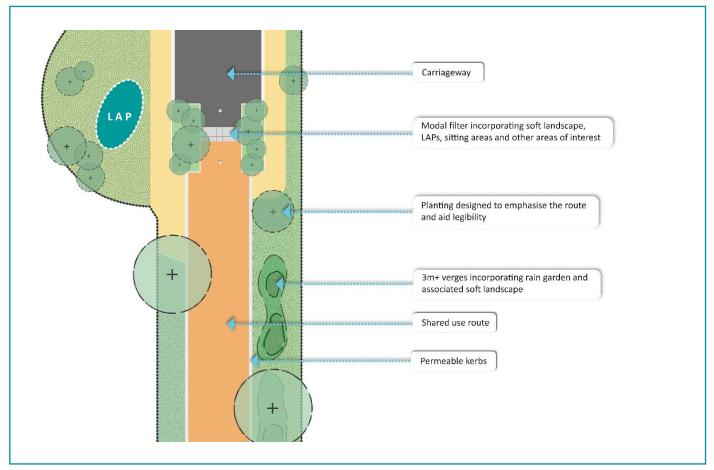
Figure 4: Illustration of an acceptable street tree layout on an Active Travel Corridor.
